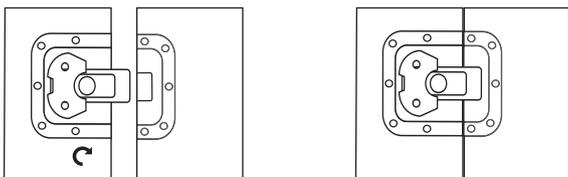
Fix the elements through the fly cases fixations by turning the clamping handle
