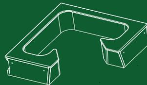
Pièce PC1 X4 (L:750mm / l: 750mm / ep:18mm)
