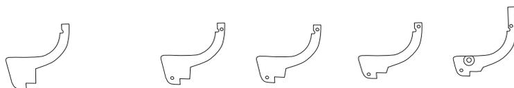
Pièce PS7 X4 (L:200mm / l: 70mm / ep:18mm)
