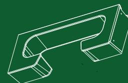
Pièce PS1 X2 (L:900mm / l: 400mm / ep:18mm)
